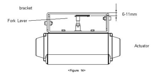
6) Attach YT-2300R to the bracket. Fix the clamping pin on the main shaft's center of YT-2300R and insert connection bar into the fork lever slot, so it can be locked to the fork lever spring. This sets the alignment of the main shaft of YT-2300R and center of the actuator stem. Bad alignment of the main shaft and the actuator stem lowers YT-2300R's durability, because too much force will be on the main shaft of YT-2300R. <Figure 15>
