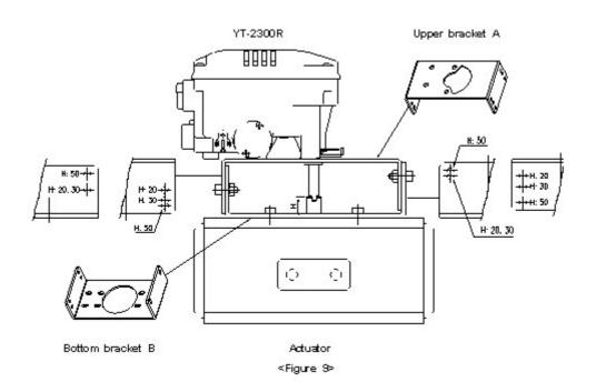
1) Standard actuator stem height (H) is 20, 30, or 50mm. After checking "H", assemble with the bracket as shown in <Figure 9, 10, & 11>
