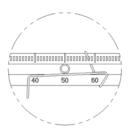
Check the valve stroke. The stroke marks are indicated on the feedback lever.
