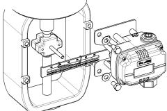
5. Connect supply pressure to the actuator temporarily. Supply enough supply pressure to the actuator in order to position the actuator clamp at 50% of the total valve stroke.
